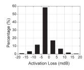
Figure 2. Histogram of activation loss. In most cases, activation loss is less than 0.01 dB.
